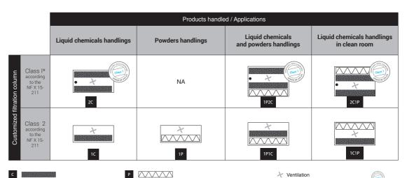
Carbon filtration for gases and vapours
