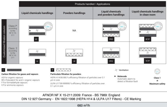
Carbon filtration for gases and vapours AS:For organic vapours
