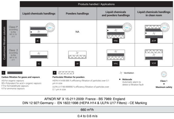
Carbon filtration for gases and vapours AS:For organic vapours
